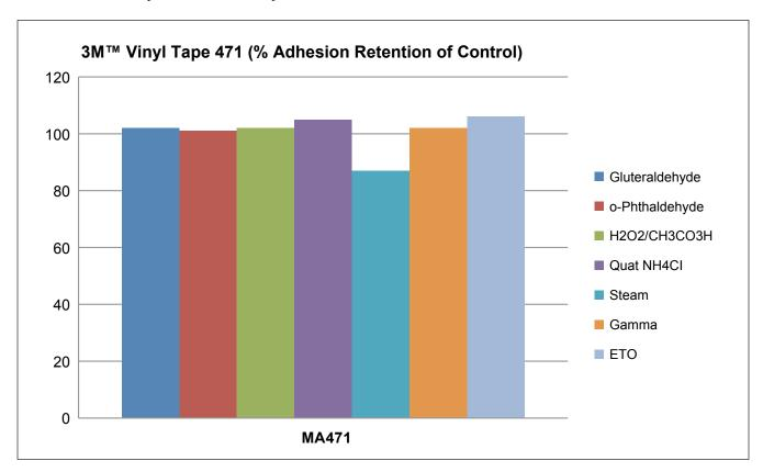
In these evaluations, performance of the tape was not negatively affected by exposure to the various sterilization methods. The product performed similar to the control sample, with all samples maintaining at least 85% of the strength of the control.
